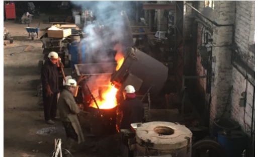
A bell being cast at John Taylors Bell Foundry - just out of interest this is one of the three new ones for St Mary's Beverley back in 2019
